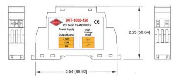
Dimensions are in inches and Millimeters
