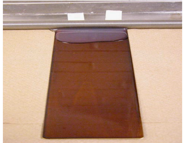
Figure 4 – Aluminum Panel with Drawdown Rod
